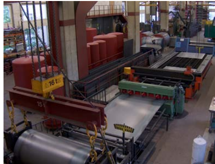
Starting from the 16-ton-steel coil, tanks are produced in series or individually
