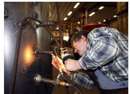
Each tank is filled with water and subjected to a strict quality control (pressure test)
