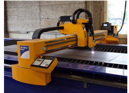
The ports are cut out of the unrolled plate by a modern plasma cutter
