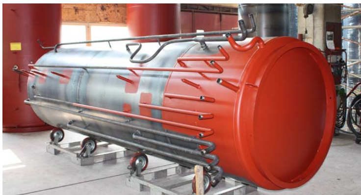
Work in progress: solar tank with welded piping
