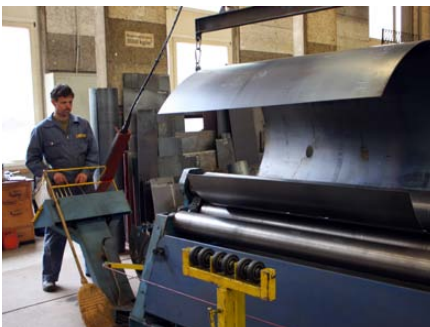
The tank shell is rounded
